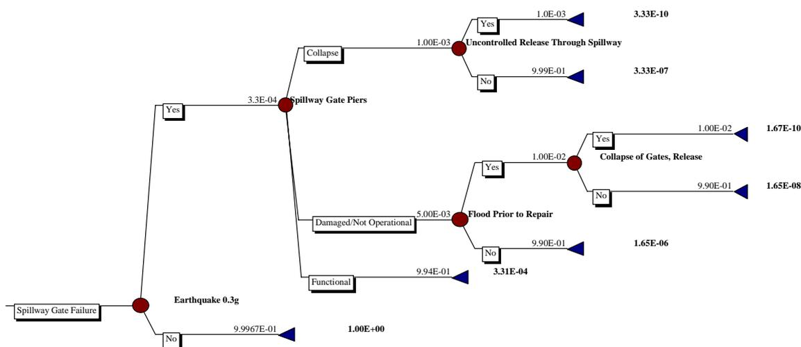
Figure 2. Typical Event Tree for Spillway Gate Failure Scenario
