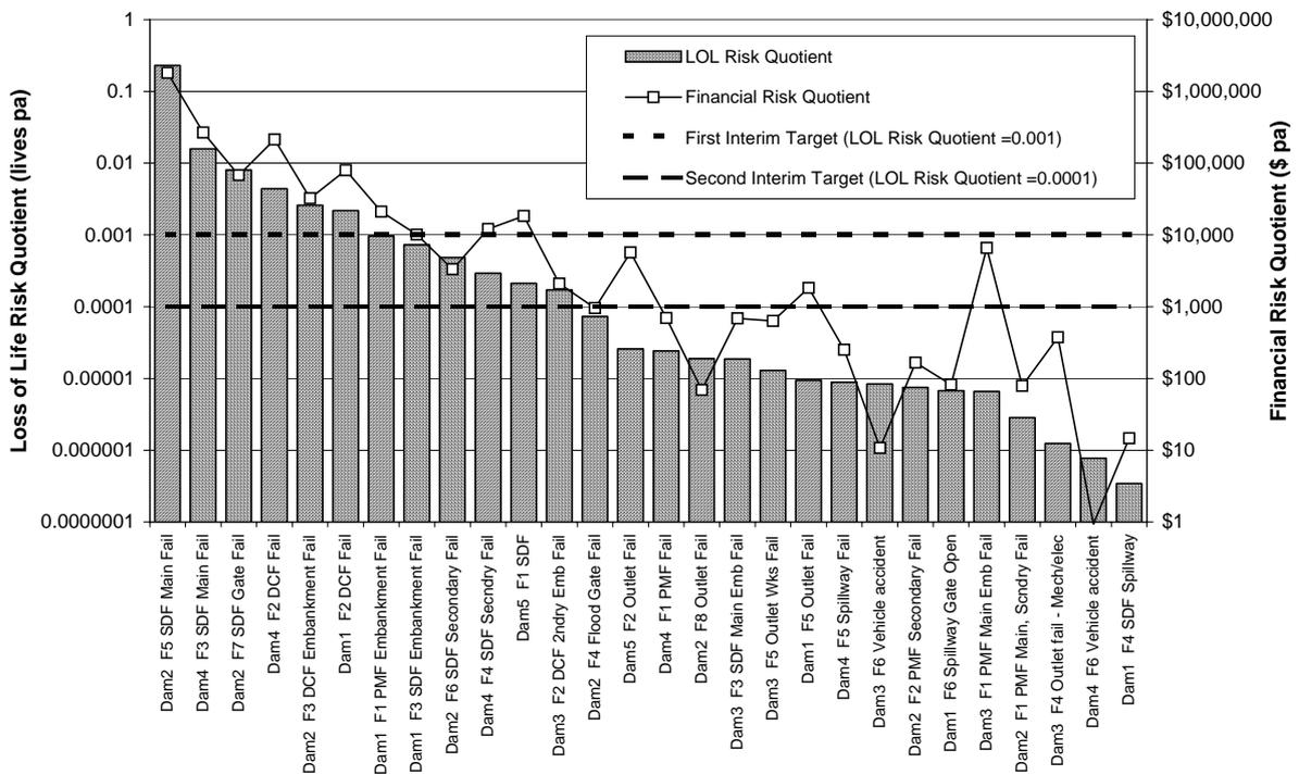
Figure 4. Risk Ranking of Failure Types
