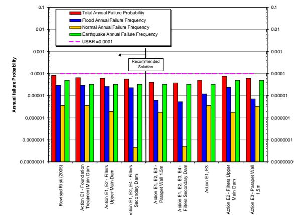
Figure 4 Existing Dam and Upgrade Options Annual Failure Probability for Loadings
