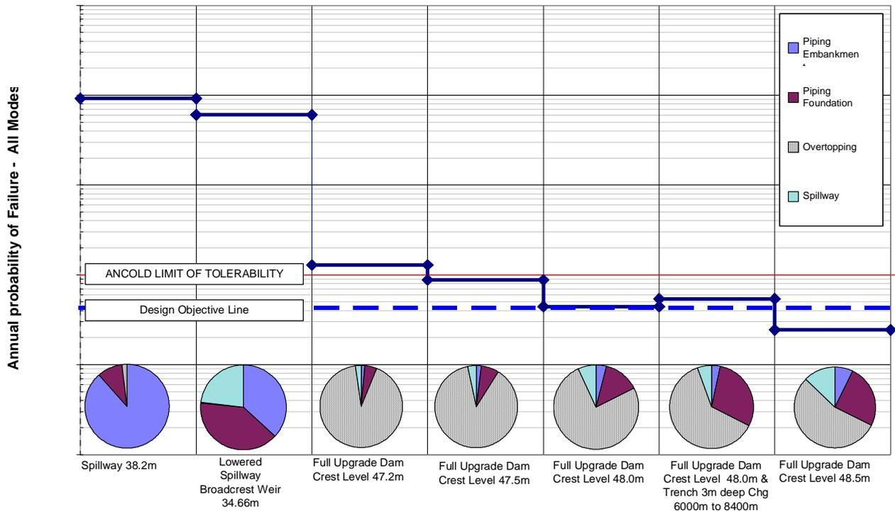
Figure 6 Dam B Total Probability of Failure for various Upgrade Options and Dam Crest Levels
